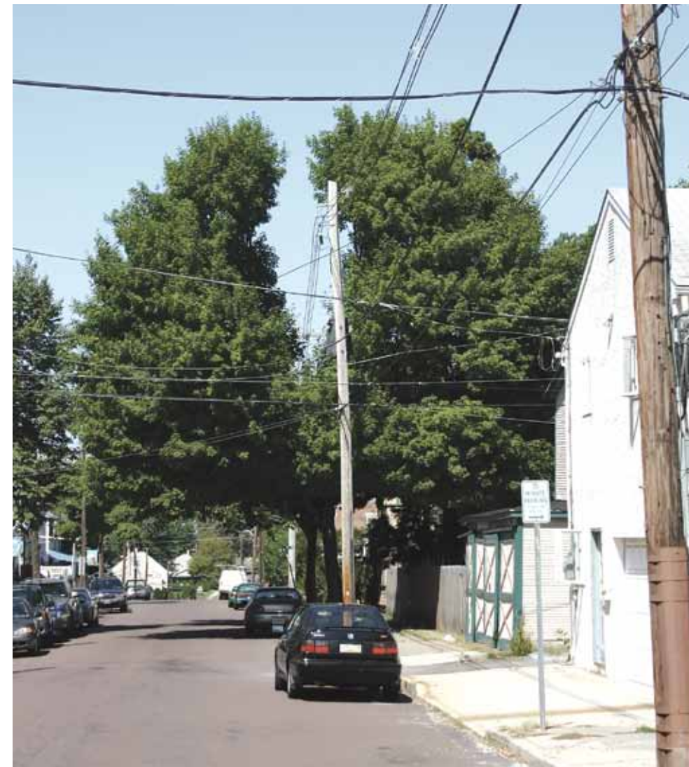
BELOW RIGHT - Thanks to bundled wiring, this maple tree is growing up and around the electric line. If there were a number of these trees in a row, the utility line would be almost invisible from the street.
