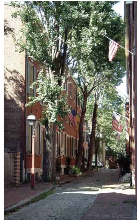
If a tree potentially grows high enough to reach its wires, PECO trims tree branches a set distance away from their wires, depending on the species of tree and the voltage running through the wires. Above, the linden trees on the left have been given a "flat top" cut more than 15 feet below the closest energized lines. Note the contrast with the appearance of the uncut linden trees on the right side of the street.
